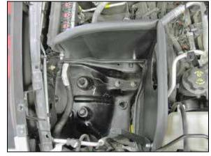
24. Install the heat shield assembly into the vehicle so that the two small "L" brackets align with the threaded stud on the inner fender and the ECU mounting stud.
