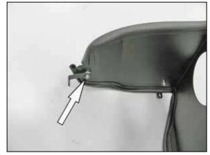
23. On 2007 vehicles, install the remaining small "L" bracket (06464) onto the heat shield with the provided spacer and hardware. NOTE: Place the spacer between the heat shield and bracket
