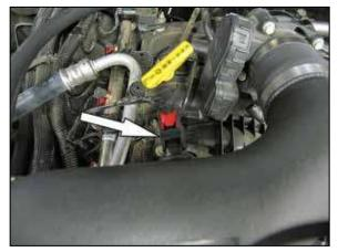
33. Reconnect the air temperature sensor electrical connection.
