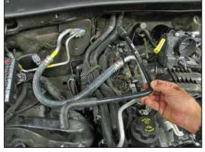
9. Unhook the crankcase vent hose from fitting on the valve cover and then remove the crankcase vent hose assembly from the vehicle.
