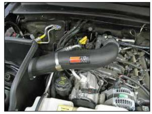
28. Install the intake tube into the silicone hose at the throttle body and align with the mounting bracket installed in step #17. Secure the tube with hose clamps provided.
