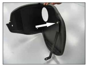
21. Install the large "L" bracket (020020) onto the heat shield and secure with the provided spacer and hardware.
