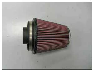
29. Install the filter adapter into the K&N® air filter and secure with the provided hose clamp. NOTE: Drycharger<sup>®</sup> air filter wrap; part # RF-1041DK is available to purchase separately. To learn more about Drycharger<sup>®</sup> filter wraps or look up color availability please visit http://www.knfilters.com<sup>®</sup>.
