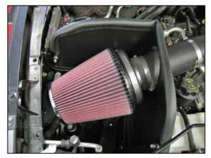
31. Install the filter assembly onto the intake tube and secure with the provided hose clamp.
