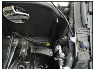
27. Secure the front heat shield mounting bracket to the inner fender with the hardware provided. **NOTE: The bolt is to be installed from under the inner fender with the large fender washer through the factory hole in the inner fender and bracket.**
