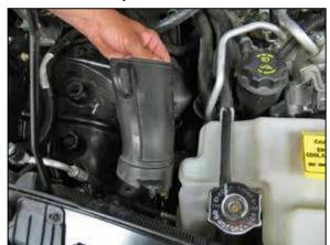
10. Remove the fresh air duct from the radiator core support as shown
