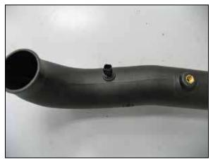
14. Install the air temperature sensor into the grommet installed in the intake tube during step #12.
