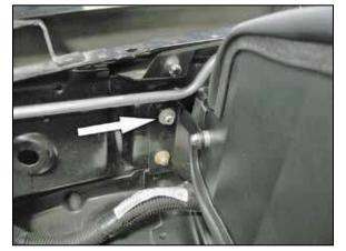
25. On 2007 model year vehicles, secure the upper heat shield mounting bracket with the nut removed in step #11.
