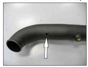
12. Install the provided grommet into the intake tube as shown.
