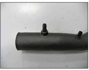
15. Install the provide  $\frac{1}{4}$  npt vent fitting into the intake tube as shown.
