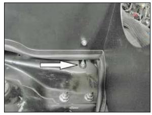
26. Secure the lower heat shield mounting bracket to the stud on the inner fender with the hardware provided.
