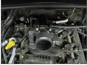
19. Install the silicone hose (08096) onto the throttle body and secure with the provided hose clamp.
