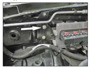
11. On 2007 model year vehicles, remove the front upper ECU mounting nut shown. **NOTE: This nut will be reused in a later step.**
