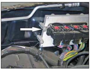
11a. On 2008 vehicles, remove the front-upper ECU mounting bolt shown. **NOTE: This bolt will be reused in a later step.**
