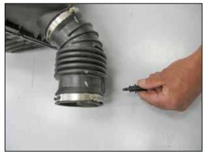
13. Remove the air temperature sensor from the stock intake tube.
