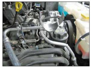
18. Install the tube mounting bracket assembly onto the A/C compressor and secure with the bolt removed in step #16.
