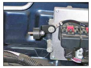
23b. On 2008 vehicles, attach the "L" bracket assembly from step #21a. to the ECU using the factory bolt removed in step #11a. **NOTE: Be sure to place the ground wire between the bracket and ECU as shown.**
