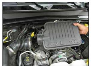
6. Remove the intake plenum from the vehicle.
