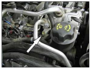
16. Remove the A/C compressor mounting bolt shown. **NOTE: This bolt will be reused.**
