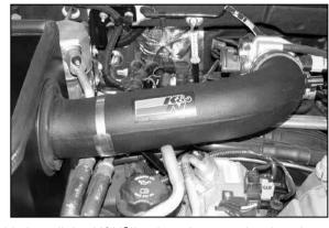
22. Install the K&N® intake tube onto the throttle body hose and position so the tube aligns with the saddle clamp. Secure with the provided hose clamps as shown.
