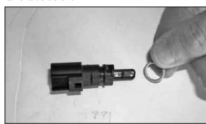
20. Remove the O-ring from the air temp. sensor as shown.
