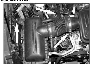
2. Loosen the hose clamp at the throttle body and the air box mounting nut, and then disconnect the crank case vent hose from the "tee" fitting.
