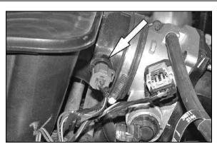
4. Depress the locking tab on the air temperature sensor electrical connection and then pull to disconnect the sensor electrical connection.
