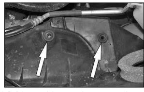
6. Pull the two-air box mounting grommets shown from the inner fender.
