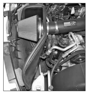
27. Install the Air filter assembly onto the K&N® intake tube and secure with the provided hose clamp as shown.
