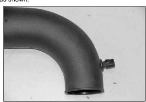
21. Install the sensor into the grommet installed in step #18.
