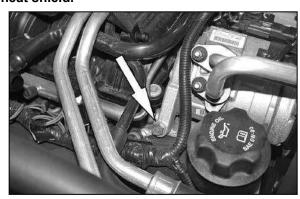
14. Remove the rear, lower A/C compressor mounting bolt shown.
