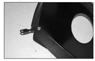
8. Install the twist bracket (070702) onto the heat shield with the provided hardware as shown.
