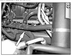
24. Install the provided silicone crank case vent hose onto the factory crank case vent tube and then onto the K&N® intake tube as shown.
