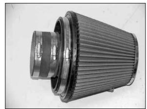
26. Install the silicone hose (08630) onto the Air filter adapter as shown and secure with the provided hose clamp as shown.
