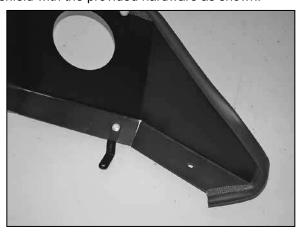
9. Install the "Z" bracket (010120) onto the heat shield with the provided hardware as shown.
