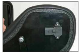
12. Install the temperature sensor onto the heat shield with the provided hardware as shown.
