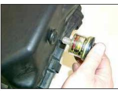
21. Remove the air filter minder and grommet from the stock air box lid as shown.
