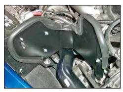
16. Install the heat shield onto the vehicle with the provided hardware.
