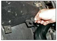
14. Install the nut insert onto the air box mounting tab as shown.
