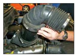
4. Remove the intake tube from the vehicle as shown.
