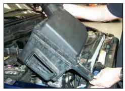
6. Remove the complete air box assembly from the vehicle as shown.
