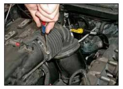
3. Loosen the hose clamps at the turbo inlet and the air box outlet as shown.
