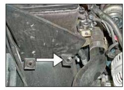
7. Remove the air box mounting grommet as shown.
