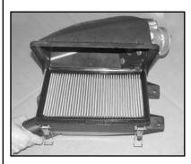
6) Install your K&N Filtercharger in the base of the airbox.
