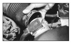
Loosen the mass air intake tube hose clamp and remove hose from mass air sensor.
