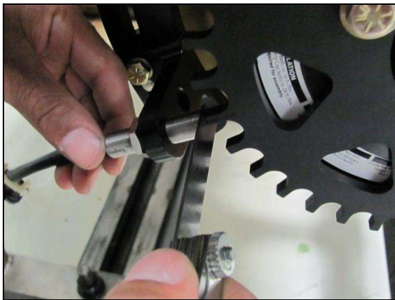
Figure 3: Adjusting the sensor gap.
