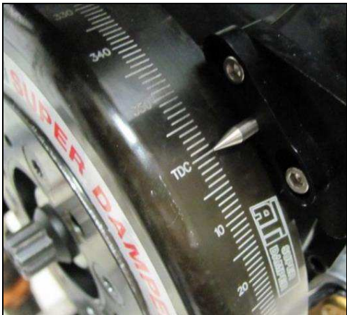
Figure 1: Rotating the engine to TDC #1.
