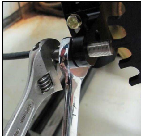
Figure 4: Locking the sensor gap.
