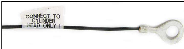
Figure 26 Coil Ground Wires
